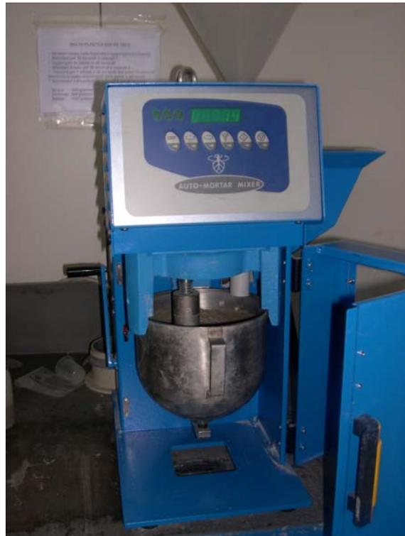
Fig. 1 - Mortar mixing apparatus UNI EN 196/1.
