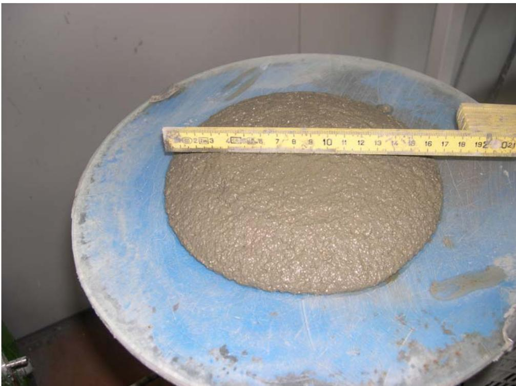
Fig. 4 A - Flow table measurement for tixotropic mortar.
