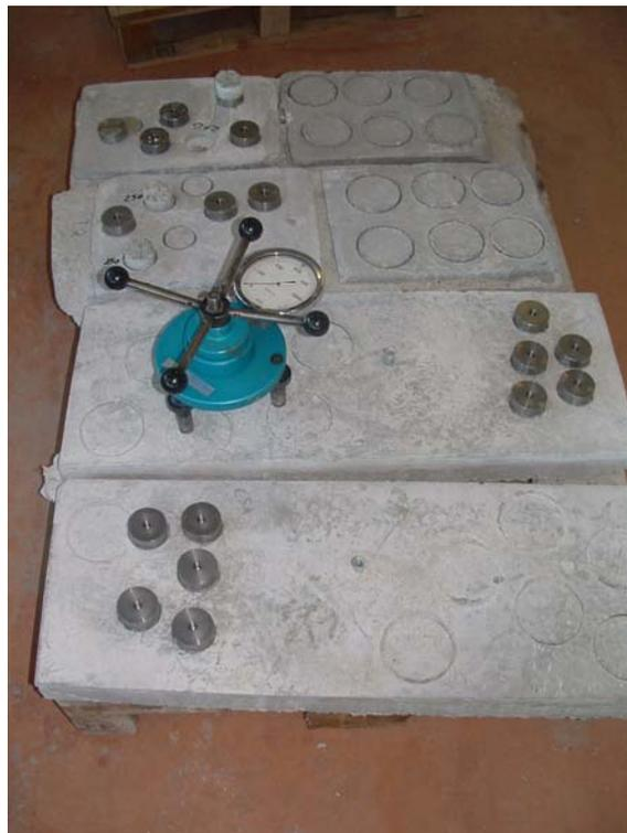
Fig. 6 - Bond strength test by pull-out (UNI EN 1542).
