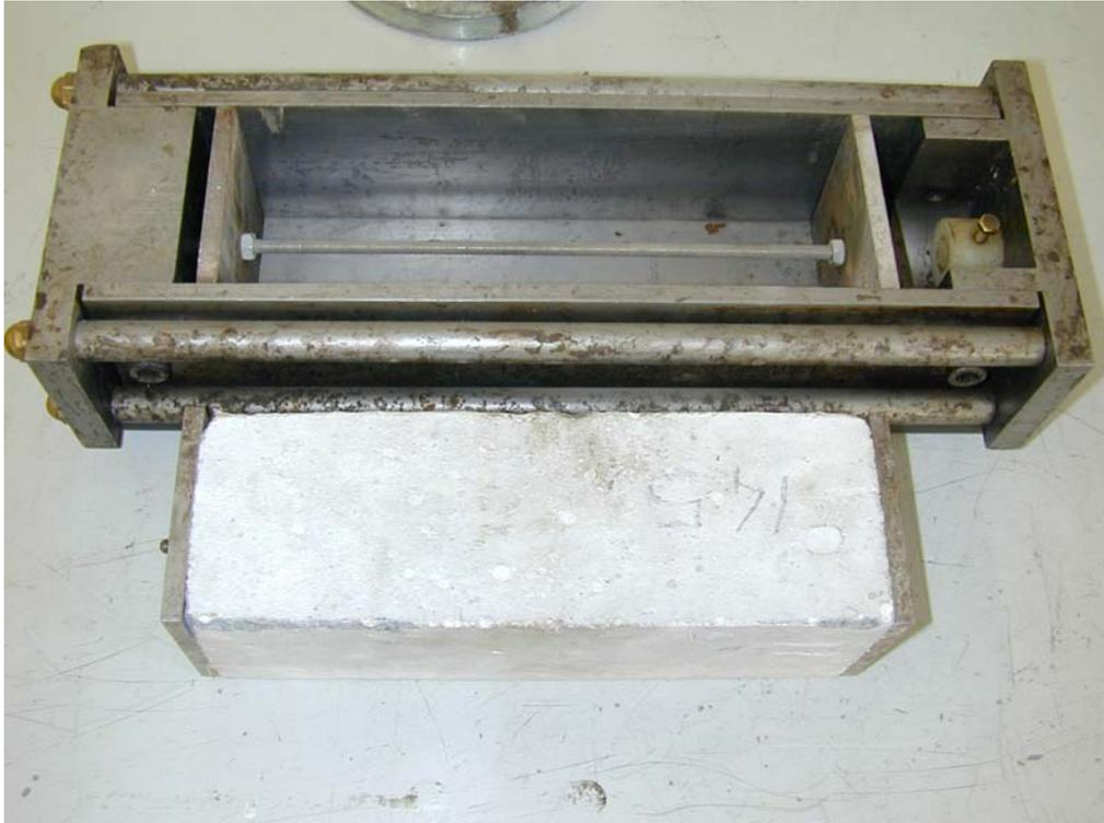
Fig. 9 - Restrained expansion specimen (UNI 8147).
