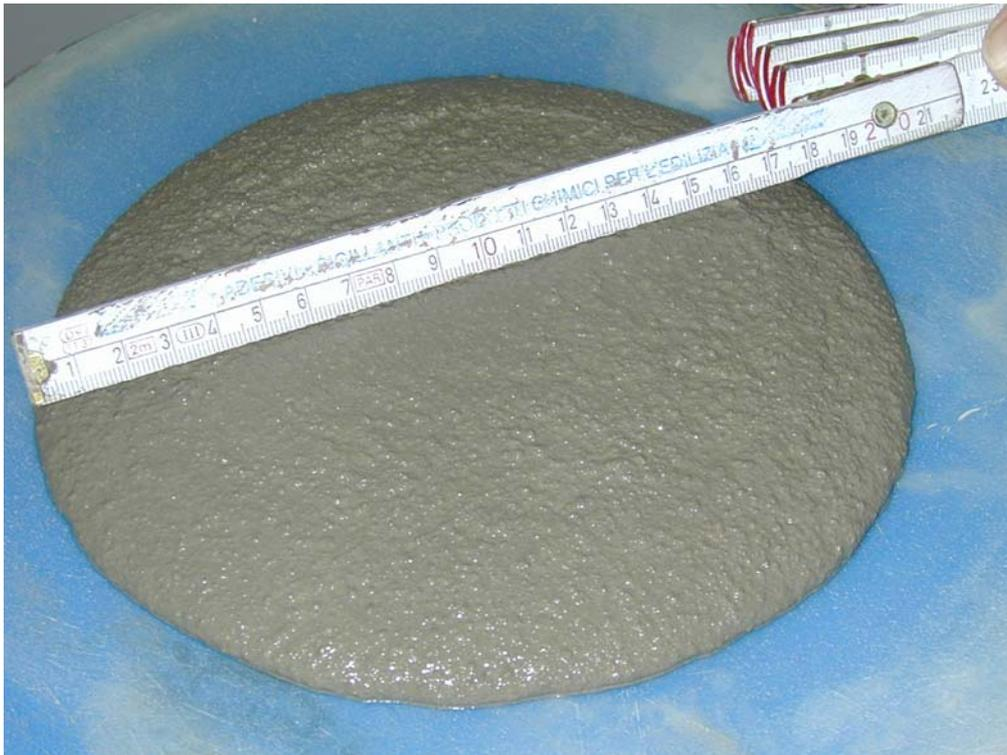
Fig. 4 B - Flow table measurement for flowing mortar.
