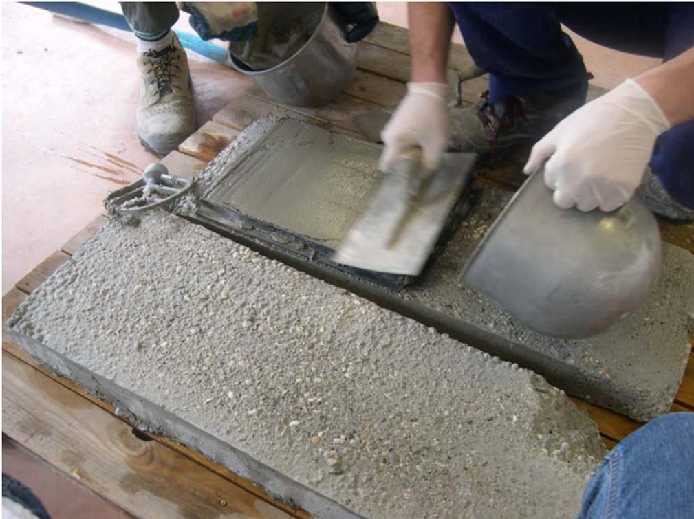
Fig. 5 - Concrete substrate for bond strength test (UNI EN 1766).
