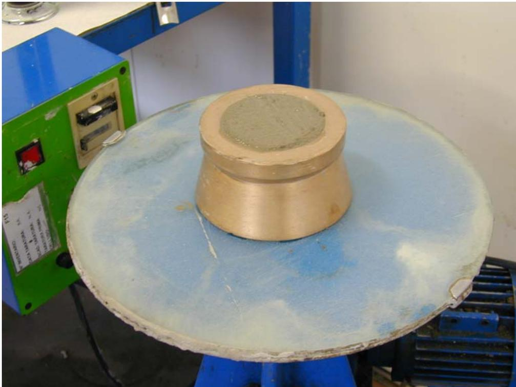
Fig. 3 - Mortar cone for flow test (UNI 7044).
