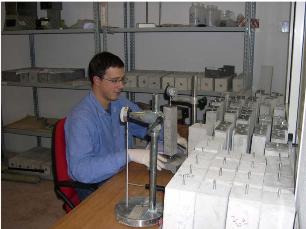
Fig. 10 - Restrained expansion measurement (UNI 8147).
