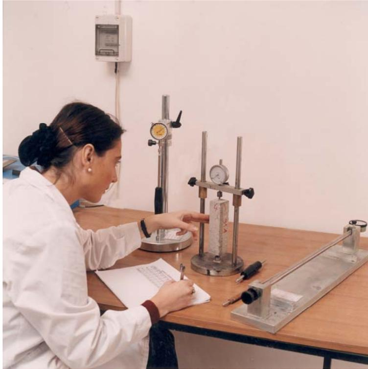
Fig. 11 - Shrinkage measurement (UNI 6687).
