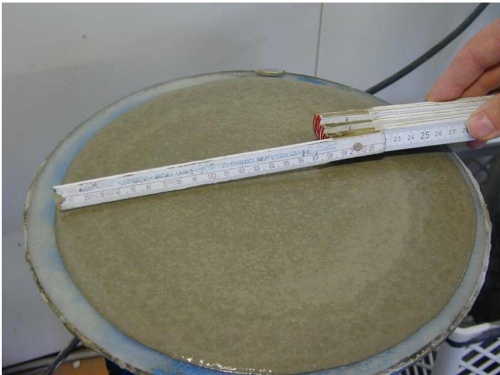
Fig. 4 C - Flow table measurement for self leveling mortar.
